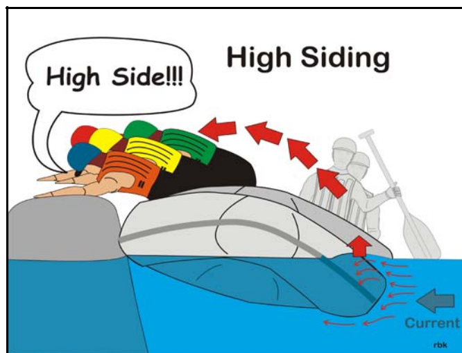
Figure 6.8: High Siding – High siding is a self-rescue technique where everyone on the upstream side moves to the downstream side of raft pinned on a rock. The strategy is that the upstream tube will float and not be pinned. Source: author – [file: \HighSide.cdr]
