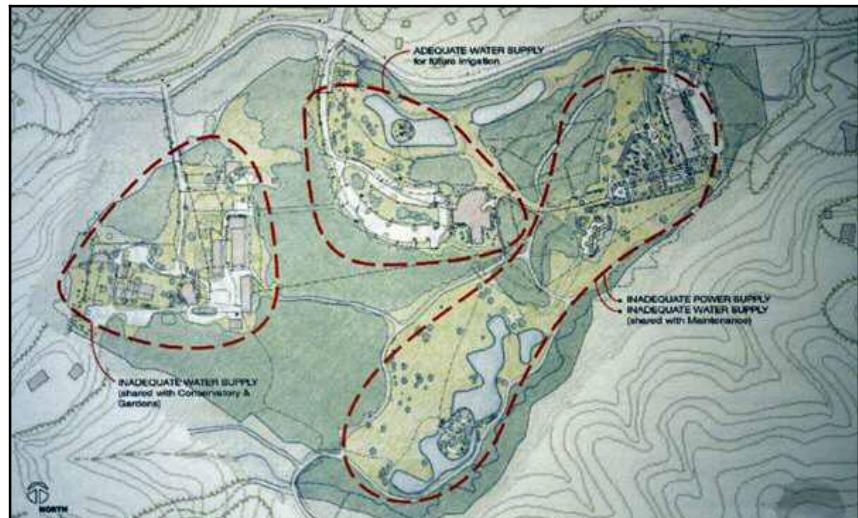
Figure 17.6 – Utilities – Brookside Gardens – Service to the major utilities is identified including water, electricity and sewage. The visitor service zone is supplied with major services. Source: 2001 Brookside Gardens Master Plan [file:\BSMP2001appx-p09utilities.pdf]
