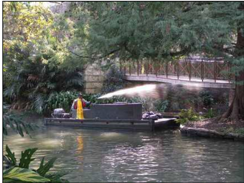
Figure 17.22 – Maintenance on the San Antonio River Walk – The original section of the River Walk in San Antonio was designed without considering maintenance. All maintenance functions including watering the plants must be done by boat. – San Antonio, Texas. Source: author – [file:\pwrpt045maintenance.pdf]
