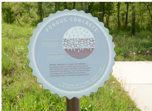
Figure 16.24: Porous Concrete – Pavements and roadways are a significant source of rain runoff. Porous concrete can allow up to five gallons of water to pass through each square foot per minute and reduce the need for retention ponds. Robinson Nature Center, Howard County, Maryland. Source: author – [file:\RNC002.jpg]
