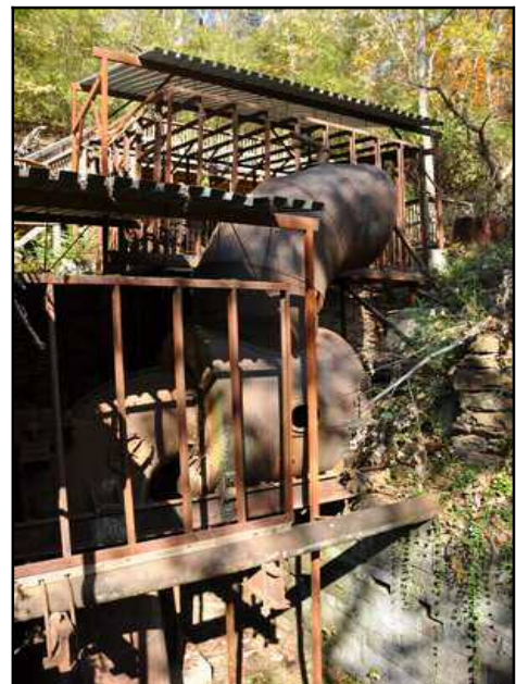
Figure 15.10 – Electric Turbine – Caption: Vandals used acetylene torches to disassemble this electric generator for its copper wire. Building a trail to the historic site along with increase visitor use has reduced additional vandalism. Roswell, Georgia. – Source: Author – [file:\Mill013.jpg]
