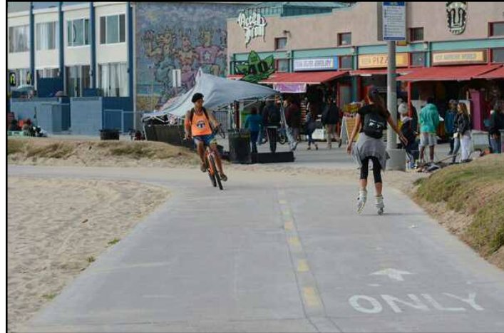
Figure 12.5: Venice Beach Special Use Trail – A “Bicycles only” sign painted on the pavement in the foreground indicates a special use trail. Reducing conflicts, both roller bladers and bicyclists travel at somewhat similar speeds. Pedestrians have the use of the promenade lined with vendors in the background. Venice Beach, California. – Source: Author – [file:\Venice236[gd].jpg]
