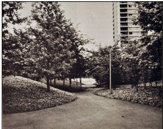
Figure 11.25: Mounding – The mounding on the left creates a physical, visual, and noise barrier. Most people will walk around the mound rather than over it. Its height blocks or limits people’s vision and it absorbs sound and limits sound transmission to primarily refracted sound. Source: Carpenter, 1975, p. 177– [file:\DSC_1008.jpg]
