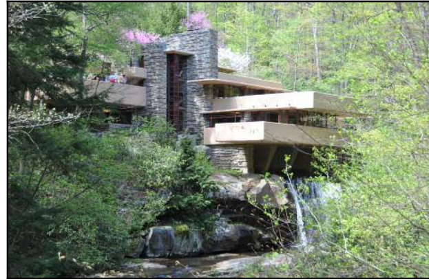
Figure 8.24: Fallingwaters – Fallingwaters illustrates the concept of asymmetry. Consider the center stone column as the center or primary axis. Although the structure on the right is larger than the structure on the left, it is offset by the structure on the left. Ohiopyle, Pennsylvania. Source: Author – [file:\FW148.jpg]
